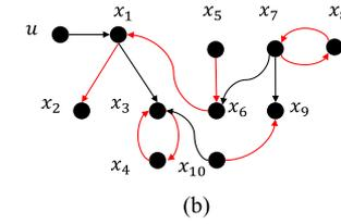
**Fig. 7.** Maximum matching  $\bar{M}$  obtained using Step 2 in Algorithm 3. In (a), we depict the system bipartite graph associated with the pair  $(\bar{A}, \bar{B})$ , whose edges are depicted in black and red (edges in red are those in the maximum matching  $\bar{M}$ ). In (b), we depict in red the edges from the system digraph  $G(\bar{A}, \bar{B})$  associated with those in the maximum matching  $\bar{M}$ .
