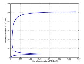
Fig. 2. The equilibria of the system given by (1). The middle range of  $T_e$ has three branches of equilibria.
