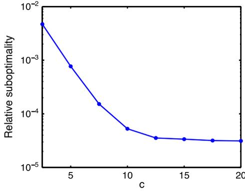
Fig. 2. Relative suboptimality of the differentially private distributed EV charging algorithm (Algorithm 2) as a function of the step size constant  $c$ . The other parameters used in the simulations are  $\epsilon = 0.1$  and  $K = 6$ .
