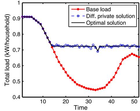
Fig. 1. Typical output of the differentially private distributed EV charging algorithm (Algorithm 2) with  $\epsilon = 0.1$  compared to the optimal solution of problem (2). The other parameters used in the simulation are  $K = 6$  and  $c = 10$ .
