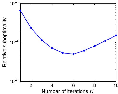
Fig. 3. Relative suboptimality of the differentially private distributed EV charging algorithm (Algorithm 2) as a function of the number of iterations  $K$ . The other parameters used in the simulations are  $\epsilon = 0.1$  and  $c = 10$ .
